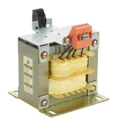
BLOCK control transformer, open core, 350 VA, 1-phase, 240/480 VAC, 24 VAC secondary, 50/60 Hz, panel mount.
