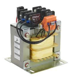
BLOCK control transformer, open core, 350 VA, 1-phase, 240/480 VAC, 120 VAC secondary, 50/60 Hz, fused, panel mount.
