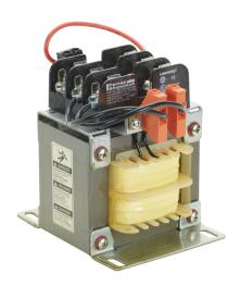
BLOCK control transformer, open core, 250 VA, 1-phase, 600 VAC, 120 VAC secondary, 50/60 Hz, fused, panel mount.
