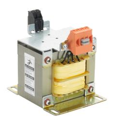
BLOCK control transformer, open core, 250 VA, 1-phase, 240/480 VAC, 24 VAC secondary, 50/60 Hz, panel mount.
