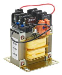
BLOCK control transformer, open core, 150 VA, 1-phase, 600 VAC, 120 VAC secondary, 50/60 Hz, fused, panel mount.
