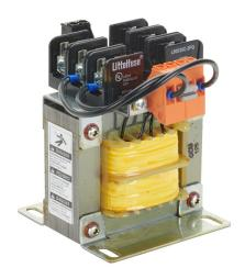
BLOCK control transformer, open core, 150 VA, 1-phase, 240/480 VAC, 120 VAC secondary, 50/60 Hz, fused, panel mount.
