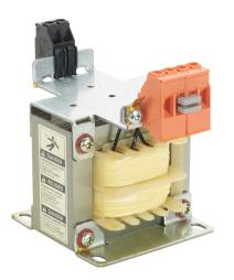
BLOCK control transformer, open core, 100 VA, 1-phase, 240/480 VAC, 24 VAC secondary, 50/60 Hz, panel mount.
