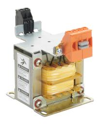
BLOCK control transformer, open core, 100 VA, 1-phase, 240/480 VAC, 120 VAC secondary, 50/60 Hz, panel mount.
