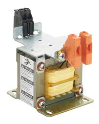
BLOCK control transformer, open core, 50 VA, 1-phase, 600 VAC, 120 VAC secondary, 50/60 Hz, panel mount.
