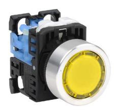
Fuji Electric pushbutton, 22mm, push ON - push OFF, LED illuminated, (1) N.O. contact(s), plastic base, metal bezel, Operator: yellow, flush, 30mm, round, plastic, 24 VAC/VDC, full voltage.
