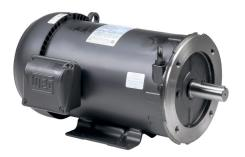
WEG Electric S premium efficiency AC induction motor, general purpose and inverter rated, 5hp, 3-phase, 208-230/460 VAC, 1800rpm, TEFC, 184TC frame, rolled steel, C-face/rigid base mount.
