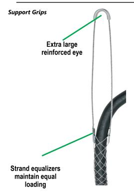
Support Grips are applied to the vertical or horizontal runs of cable or service lines to support dead weight and reduce potential damage due to breakage or stress. These grips are designed to be used indoors for cable support where flexible cable connects electrical equipment to bus duct. Applications also include support for air hoses and water hoses.
