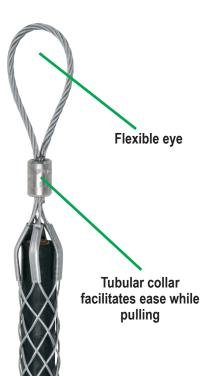
Pulling Grips are designed to serve as reusable tools for light industrial pulling of electrical cable and for underground and industrial plant wiring and re-wiring. These grips offer protection from abrasion and ease the cable through bends and rough surfaces. They also serve as a temporary splice, when replacing old cable with new, and to pull slack in new construction or maintenance operations.
