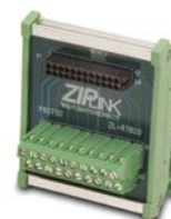
ZL-RTB20 20-pin feed-through connector module
