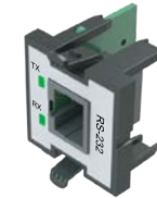
BX-P-SER2-RJ12 RS-232 Port (RJ12)
