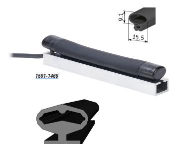
The SENTIR edge safety contact edges of ASO Safety Solutions are pressure-sensitive sensors applied to ensure the safety of closing edges at possible crushing or shearing points which are prone to accidents. They may be installed near automatic gates, machines and other facilities for handling equipment or moving stage elements in order to protect individuals from bodily harm or machinery from damage.
