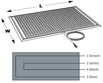
Use wire leads brown and white (1 & 2) for channel 1. Use wire leads blue and black (3 & 4) for channel 2. The channels should have continuity when pressure is applied to the mat.
