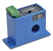
DCS100 series current switches combine a Hall effect sensor, signal conditioner and limit alarm into a single package for use in DC current applications up to 100A. The DCS100 series has jumperselectable current input ranges and your choice of Normally Open Solid-State or SPDT Relay outputs. This series is available in fixed core models only.
