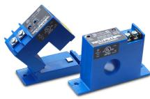
ACS150 Series current operated switches combine a current transformer, signal conditioner and limit alarm into a single package for use in monitoring or proof of operation applications. Offering an adjustable setpoint range of 1 to 150 amps and universal, solidstate outputs, the self-powered ACS150 can be tailored to provide accurate and dependable digital indication of overcurrent conditions across a broad range of applications. The ACS150 is available in fixed-core and split-core models.
