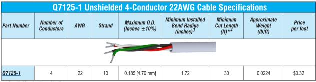
1. Installed bend radius ≥ 10x diameter
