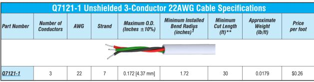
1. Installed bend radius ≥ 10x diameter
