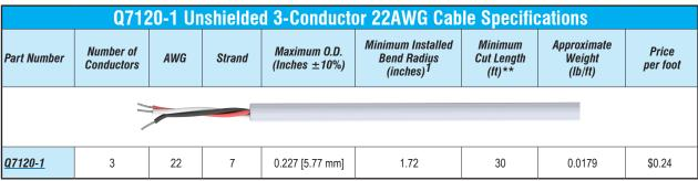
1. Installed bend radius ≥ 10x diameter
