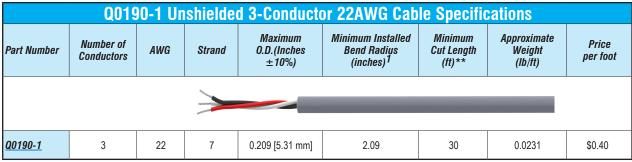
1. Installed bend radius ≥ 10x diameter
