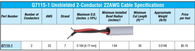
1. Installed bend radius ≥ 10x diameter
