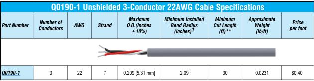
1. Installed bend radius ≥ 10x diameter
