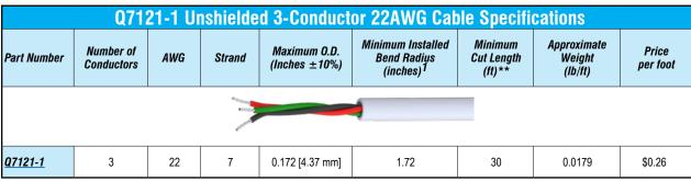
1. Installed bend radius ≥ 10x diameter
