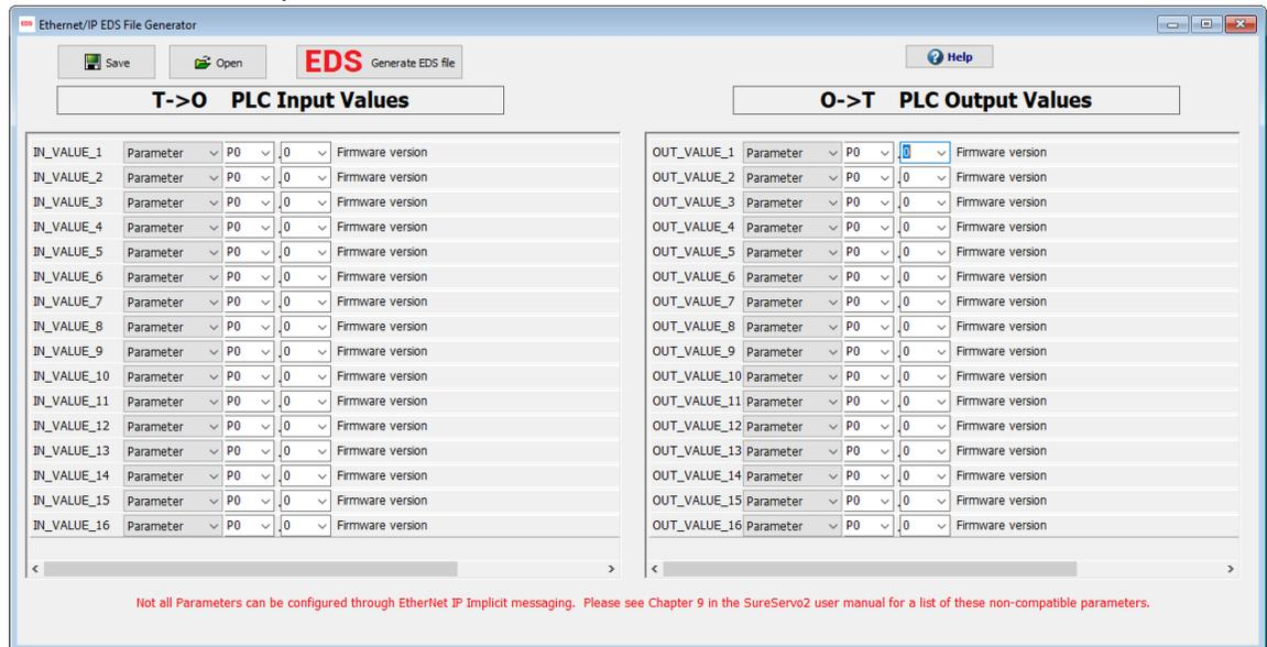
If your PLC supports EDS files, it will be able to import the EDS file into the PLC configuration software.
