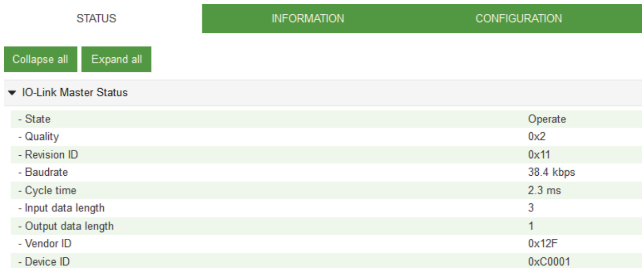
Fig. 10-9: IO-Link master port – IO-Link master status
