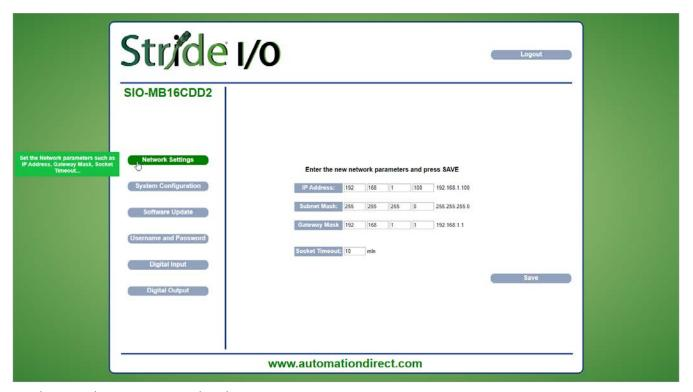
On the Network Settings page, set the Ethernet communication parameters.
