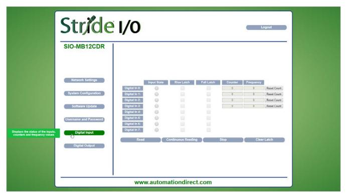
This page displays the state of the digital inputs and their associated latches.
