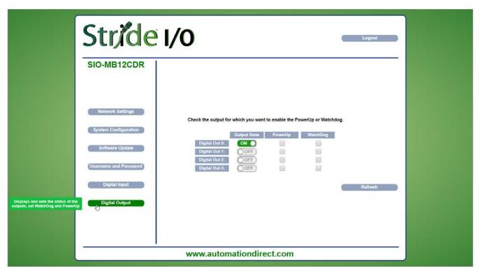
This page displays the values of and allows writing to the digital outputs, and allows configuration of the PowerUp and Watchdog settings for each output.
