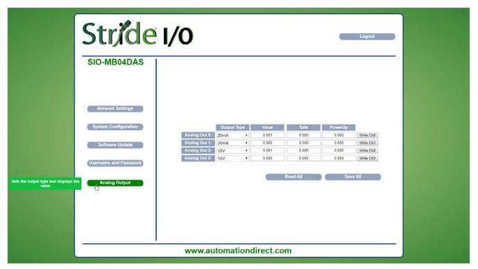
This page displays the values of and allows writing to the analog outputs in the unit of measurement defined by the "Output Type". Each Output can be configured independently as voltage or current. Each output is electrically isolated from all others.
