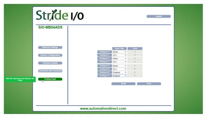
The four analog input channels are electrically isolated from each other. Each channel supports one voltage and one current input that may be used simultaneously.
