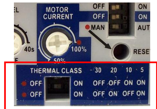
Figure 7 – Thermal Class Dip Switch Location
