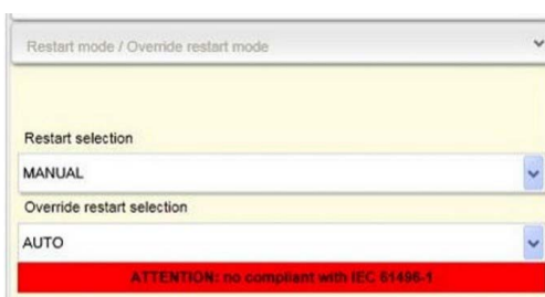
Figure 42 - ACM Configuration: Auto Override Restart Selection
