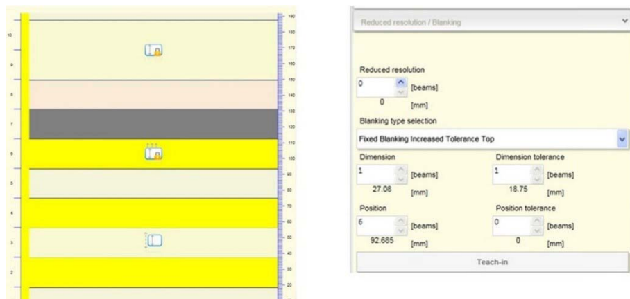
Figure 59 - Fixed Blanking with increase tolerance
