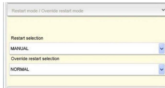
Figure 44 - ACM Configuration: Normal Override Restart Selection
