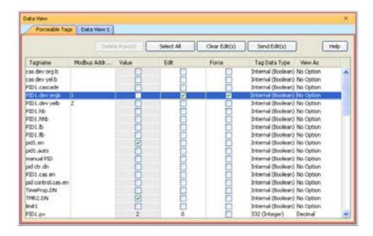
From either of these windows you have the option to select the check box in the Force column. When this box is checked and the row is selected (selected rows show highlighted blue) and you select the Send Edit(s) button, the current row(s) will be forced.
