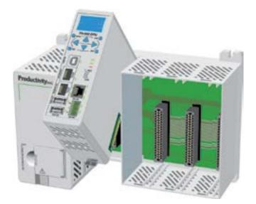
3. Install I/O Modules and engage locking tabs.
