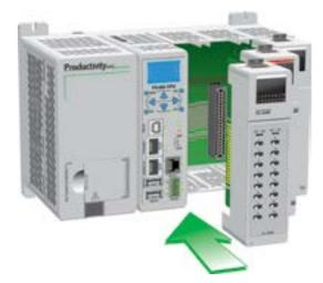
4. Connect appropriate wiring to power supply and I/O, a P3-01AC and P3-08TAS in this example.
