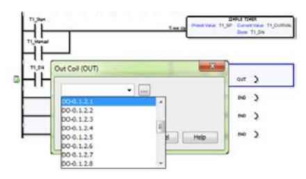
The ladder program now looks like this. When either of the T1 contacts are energized, the timer starts. When it times out, contact T1\_DN energizes and turns on the rung 2 output.
