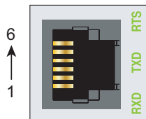
6-pin RJ12 Female Modular Connector
