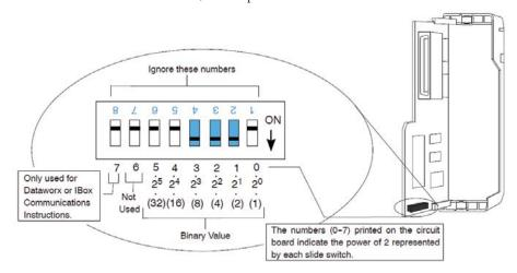
The Module ID equals the sum of the binary values of the slide switches set in the ON position. For example, if you set slide switches 1, 2, and 3 to the ON position, the Module ID will be 14. This is found by adding 8+4+2=14. The maximum value you can set on the DIP switch is 32+16+8+4+2+1=63. This is achieved by setting switches 0 through 5 to the ON position.
