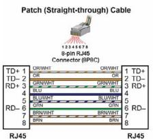
The above diagrams illustrate the standard wire positions in the RJ45 connector. We recommend all ECOM 10/100BaseT cables to be Category 5, UTP cable.
