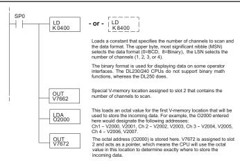
The following tables show the special V-memory locations used by the D2-240, D2-250-1, D2-260 and D2-262 for the CPU base and local expansion base I/O slots. Slot 0 (zero) is the module next to the CPU or D2-CM module. Slot 1 is the module two places from the CPU or D2-CM, and so on. Remember, the CPU only examines the pointer values at these locations after a mode transition. Also, if the D2-230 (multiplexing) method is used, verify that these addresses in the CPU are 0 (zero).
