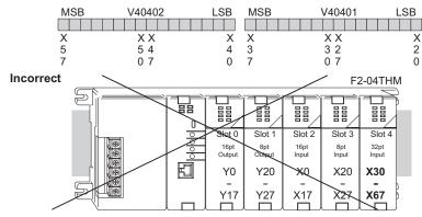
Data is split over three locations, (see graphic below) so instructions cannot access data from a D2-230 CPU.
