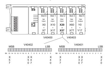
When a D2-230 CPU is used, the input points must start on a V-memory boundary. To use the V-memory references required for a D2-230 CPU, refer to the table below. The first input address assigned to a module must be one of the X inputs shown. The table also shows the V-memory addresses that correspond to these X inputs.
