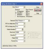
**Step 2:** In *Direct*SOFT, open a Data View window and type in the special V-memory locations used for the DCM module based on the slot the module is occupying (see page 3–9). The BCD/HEX register values needed to support your specific port communications selections will be displayed in the Data View window.
