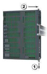
1. Fully extend the three mounting tabs located on the top and bottom of the unit.
