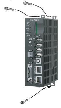
2. Secure to a panel using three #8 standard or M4 metric screws and appropriate hardware.
