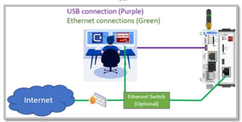
Ethernet Only\* — Connect your PC, and each Ethernet enabled module to a switch. All modules can be accessed over the same network and all will have access to HTTP services. If you have multiple network adapters on your PC (Wi-Fi and Wired, or multiple wired), you will not be able to connect one adapter to an external network (Internet) and the second adapter to the C2-NRED module. Node-RED will not communicate across bridged adapters or shared connections.
