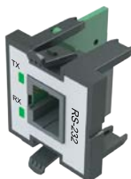
BX-P-SER2-RJ12 RS-232 Port (RJ12)
