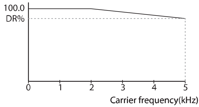
Continuous rated current for light load
