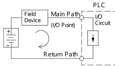
If there was unlimited space and budget for I/O terminals, then every I/O point could have two dedicated terminals. However, providing this level of flexibility is not practical or even necessary for most applications. So, most input or output points on PLCs are in groups that share the return path (called *commons*). The figure at the right shows a group (or bank) of four input points that share a common return path. In this way, the four inputs require only five terminals instead of eight.
