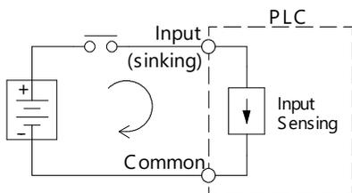
**Sinking** = provides a path to supply common (-)
