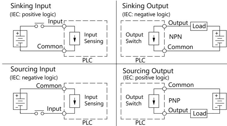
Sink/source I/O circuits combine sinking and sourcing capabilities. This means that the I/O circuitry in the PLC will allow current to flow in either direction, as shown at the right. The common terminal connects to one polarity, and the I/O point connects to the other polarity (through the field device). This provides flexibility in making connections to your field power supply. Please note:
