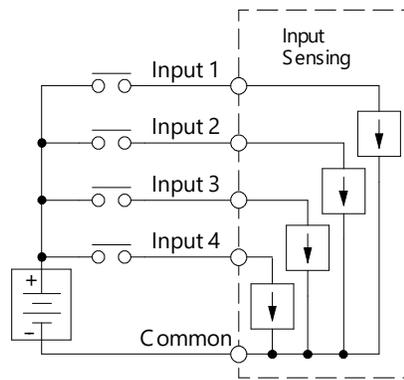
**NOTE:** Assuming all input circuits have a similar resistance, the current at the common terminal is four times greater than the current at any one of the inputs. This effect is especially important to note for output circuits, where the current through a common terminal can reach several amperes. You will need to decide whether to fuse each output point individually, or to put a fuse in the common terminal path.
