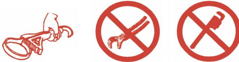
**Attention:** Proper care must be taken while installing this or any plastic threaded valve into a piping system, or failure of the valve body may occur.
