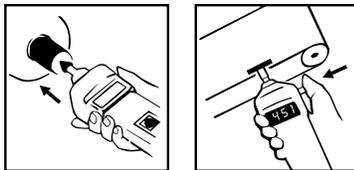
Apply only enough pressure to eliminate slip. A blinking red dot appears on the upper right corner of the display when shaft is turning.
