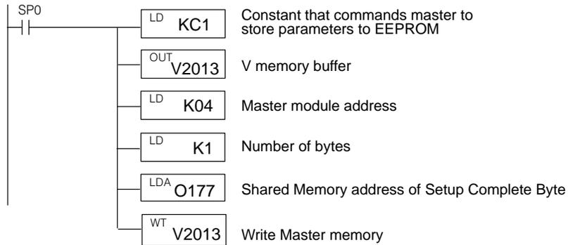
We can now complete the setup program. This last block of logic tells the remote master to save the parameters in EEPROM (setup is complete). The setup complete logic structure is the same for any channel using a D2-RMSM as a master.
