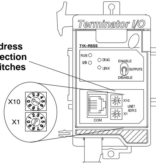
One switch is marked X1 and the other X10. Don't confuse these with the conventional data type labeling – *these do not refer to inputs X1 and X10*. Instead, these set the address in decimal for each unit. X1 is the “one's” position and X10 is the “ten's” position. For example, set address 7 by turning the X10 switch to 0 and the X1 switch to 7.
