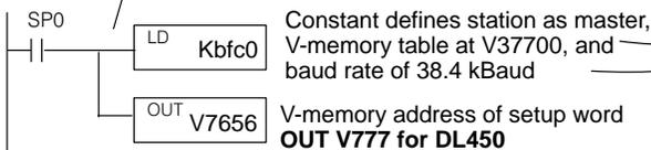
Constant defines station as master, V-memory table at V37700, and baud rate of 38.4 kBaud
