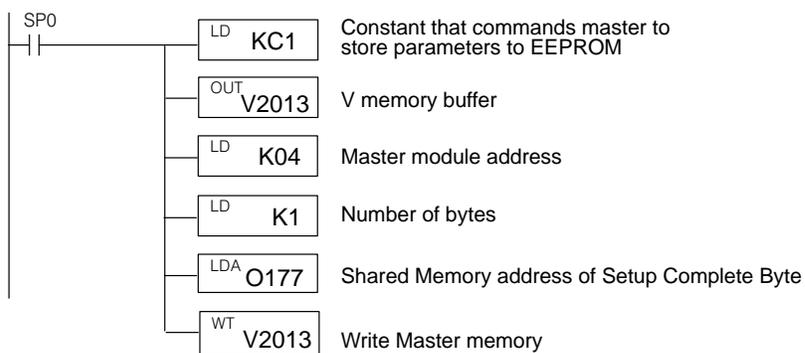
We can now complete the setup program. This last block of logic tells the remote master to save the parameters in EEPROM (setup is complete). The setup complete logic structure is the same for any channel using a D2-RMSM as a master.
