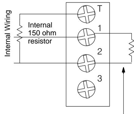
You add your own resistor, using a resistor between 100 and 500 ohms.
