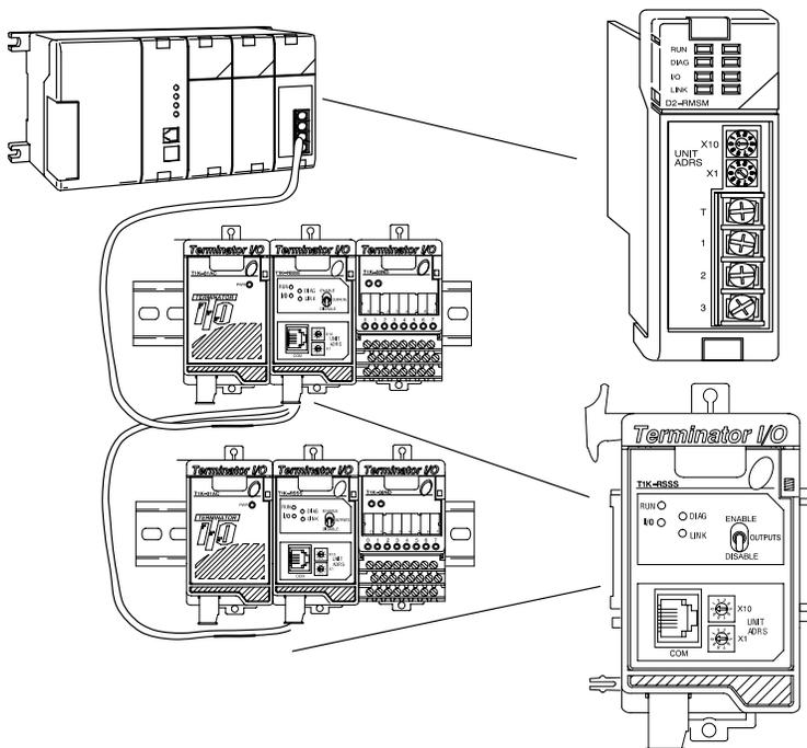
**Remote Master :** The master module(s) are mounted in the CPU base.
