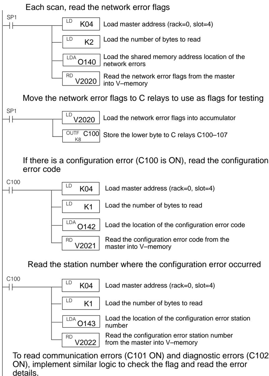
You can then use the retrieved data in logic or display it in a Dataview in **DirectSOFT** to determine the nature and location of the error. The Network Error Table describes the error codes.
