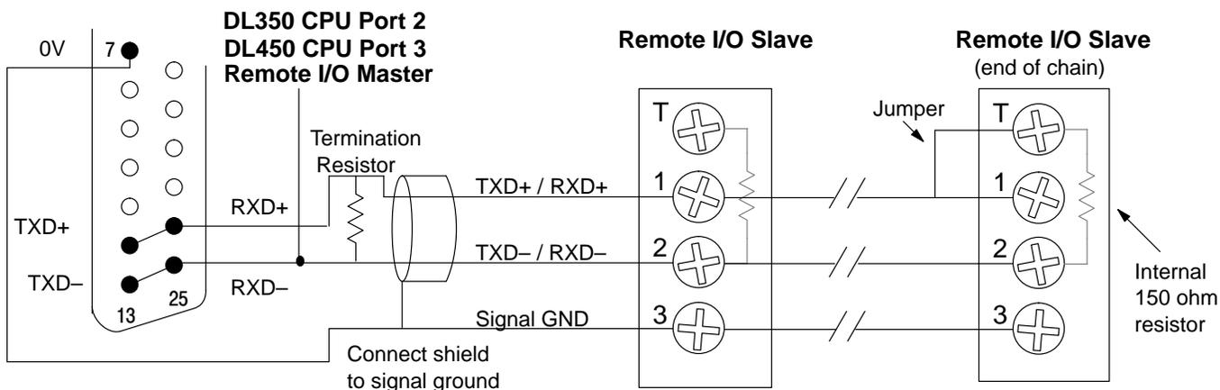
The twisted/shielded pair connects to the DL350/DL450's Port as shown. Be sure to connect the cable shield wire to the signal ground connection. A termination resistor must be added externally to the CPU, as close as possible to the connector pins. Its purpose is to minimize electrical reflections that occur over long cables. Be sure to add the jumper at the last slave to connect the required internal termination resistor.
