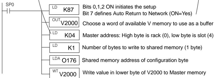
This block of logic tells the remote master the starting V-memory addresses for the inputs and outputs, and the total number of each for the channel. Use the LD, LDA, and OUT commands to load the starting addresses and point totals into temporary memory, then write the values to the master's shared memory. The Quick Reference Table shows the correct shared memory addresses in octal.
