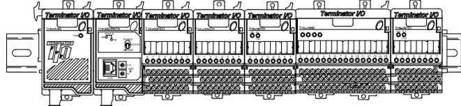
Based on the V-memory addresses we chose, the D2-RMSM allocated points X40 to X77 to Remote Slave #1's inputs, and Y40 to Y117 to its outputs. This means the starting address for the *second remote base inputs* is X100 (assigned automatically by the remote master) and the starting address for *outputs* is Y120 (assigned automatically).
