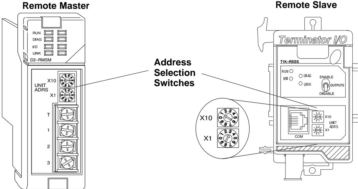
One switch is marked X1 and the other X10. Don't confuse these with the conventional data type labeling – *these do not refer to inputs X1 and X10*. Instead, these set the address in decimal for each unit. X1 is the “one's” position and X10 is the “ten's” position. For example, set address 13 by turning the X10 switch to 1 and the X1 switch to 3 ( $10+3=13$ ).
