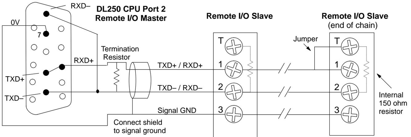
The twisted/shielded pair connects to the DL250's Port 2 as shown. Be sure to connect the cable shield wire to the signal ground connection. A termination resistor must be added externally to the CPU, as close as possible to the connector pins. Its purpose is to minimize electrical reflections that occur over long cables. Be sure to add the jumper at the last slave to connect the required internal termination resistor.
