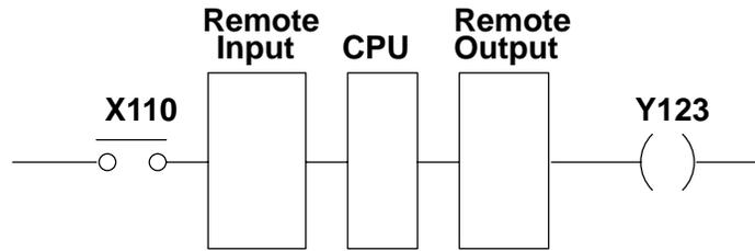
The drawing below shows the details of the CPU and Remote Master interaction .
