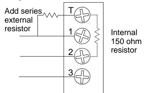
**Cabling Between the D3-350/D4-450 CPU Bottom Port and Slaves**
