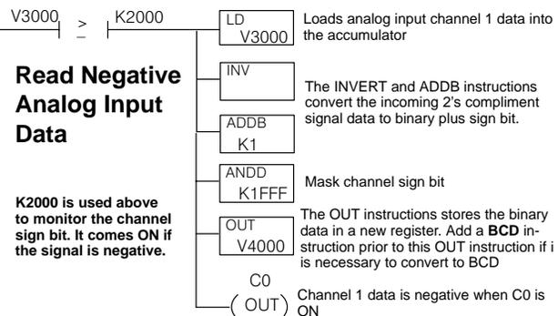
K2000 is used above to monitor the channel sign bit. It comes ON if the signal is negative.
