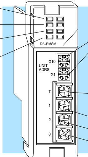
**UNIT ADRS**--Rotary switches for setting the module to be the master – **always set to 0**
