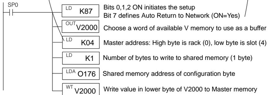
This block of logic tells the remote master the starting V-memory addresses for the inputs and outputs, and the total number of each for the channel. Use the LD, LDA, and OUT commands to load the starting addresses and point totals into temporary memory, then write the values to the master's shared memory. The Quick Reference Table shows the correct shared memory addresses in octal.
