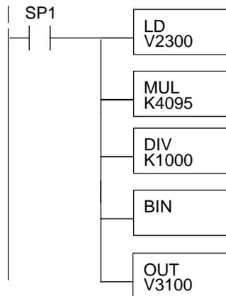
The LD instruction loads the engineering units used with channel 1 into the accumulator. This example assumes the numbers are BCD. Since SP1 is used, this rung automatically executes on every scan. You could also use an X, C, etc. permissive contact.
