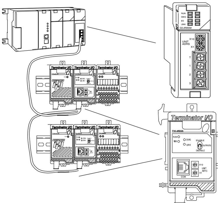
**Remote Master :** The master module(s) are mounted in the CPU base.
