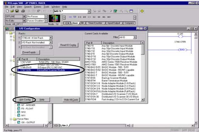
The **Advanced I/O Configuration** window will appear. The **M0** and **M1** Lengths will show the default of 256. Change this to 361.
