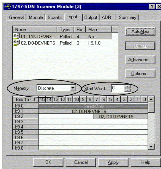
At the completion of the input AutoMapping, the window will look like this example. The T1K-DEVNETS node is now shown.
