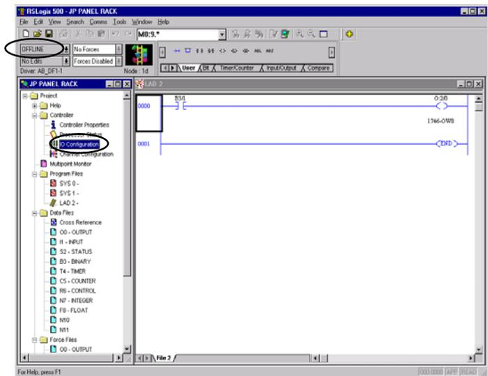
The I/O Configuration window will come into view. When you select the scanner module, verify that it is in the correct slot.
