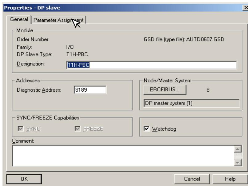
In the window **Parameter Assignment** window, click on **Hot-Swap Mode**. Auto will appear in the **Value** row opposite the selection. Click on the down arrow for a drop-down window to appear so that Manual can be selected. Click on **OK**. The T1H-PBC is now in the manual Hot-Swap Mode.
