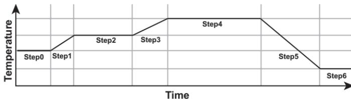
You can select which Ramp / Soak pattern the SOLO controller will execute first. The Ramp / Soak patterns can be executed in series, so the Ramp / Soak control can execute up to 64 steps (8 steps x 8 patterns). You can select which Ramp / Soak pattern will execute next or the controller stops after executing the current pattern. The SOLO controller can execute the same Ramp / Soak pattern up to 200 times before it stops or moves to the next Ramp / Soak pattern.
