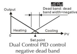
For On / Off type control the Dead Band parameter defines the area around the SV where the output remains off. The PV must go beyond the dead band range in order for either output 1 or output 2 to turn on.
