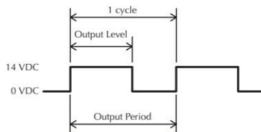
For example, when the Output Level is 60% and the Output Period is 10 seconds, the Voltage Pulse output is turned on for 6 seconds in the cycle.
