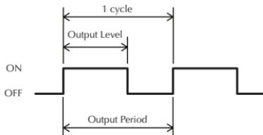
For example, when the Output Level is 60% and the Output Period is 10 seconds, the output relay is turned on for 6 seconds in the cycle.
