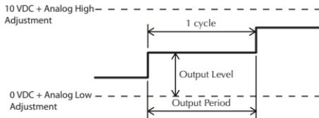
The Analog High Adjustment value may be changed to adjust the output voltage when the Output Level is 100%. The adjustment needs to be done in the Manual mode.
