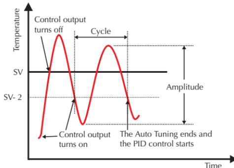
Once the Auto Tuning process is completed, the SOLO controller calculates the above PID parameters for the currently selected group (**P<sub>Ld0</sub>** - **P<sub>Ld3</sub>**) and starts the PID control with the new parameter values immediately.
