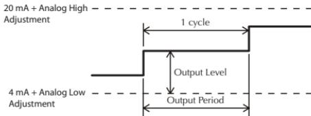
The Analog High Adjustment value may be changed to adjust the output current when the Output Level is 100%. The adjustment needs to be done in the Manual mode.
