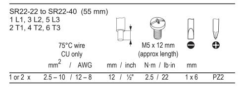
Where several conductors are to be connected, the difference between the wires/cables used must not exceed one DIN Standard size level.
