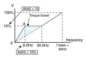
addition to the standard straight V/f line (constant torque curve).
