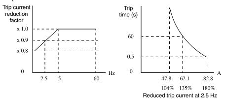
**Free Thermal Characteristic** - It is possible to set the electronic thermal characteristic using a free-form curve defined by three data points, according to the table below.
