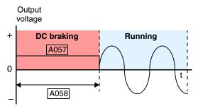
tion. If an inverter is started into such a backward-rotating load, over-current trips can occur. Use DC braking as an "anti-windmilling" technique to stop the motor and load, and allow a normal acceleration from a stop. See also the "Acceleration Pause Function" on page 3–21.
