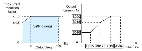
Suppose the electronic thermal setting (B012) is set to 44 Amperes. The left graph below shows the effect of the free setting torque characteristic curve. For example, at (B017) Hz, the output current level to cause overheating in a fixed time period is reduced by a factor of (B018). The right graph below shows the reduced trip current levels in those conditions for given trip times.
