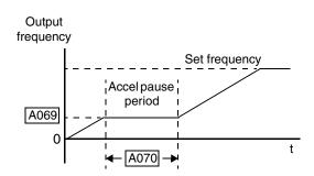
direction while the inverter is in a Stop mode. Initiating a normal acceleration in such a situation may result in over-current trips. This function can be used to keep the inverter output frequency and voltage at low levels long enough to bring the load to a stop, and commence turning in the desired direction before the acceleration ramp resumes. See also "DC Braking Settings" on page 3–18.
