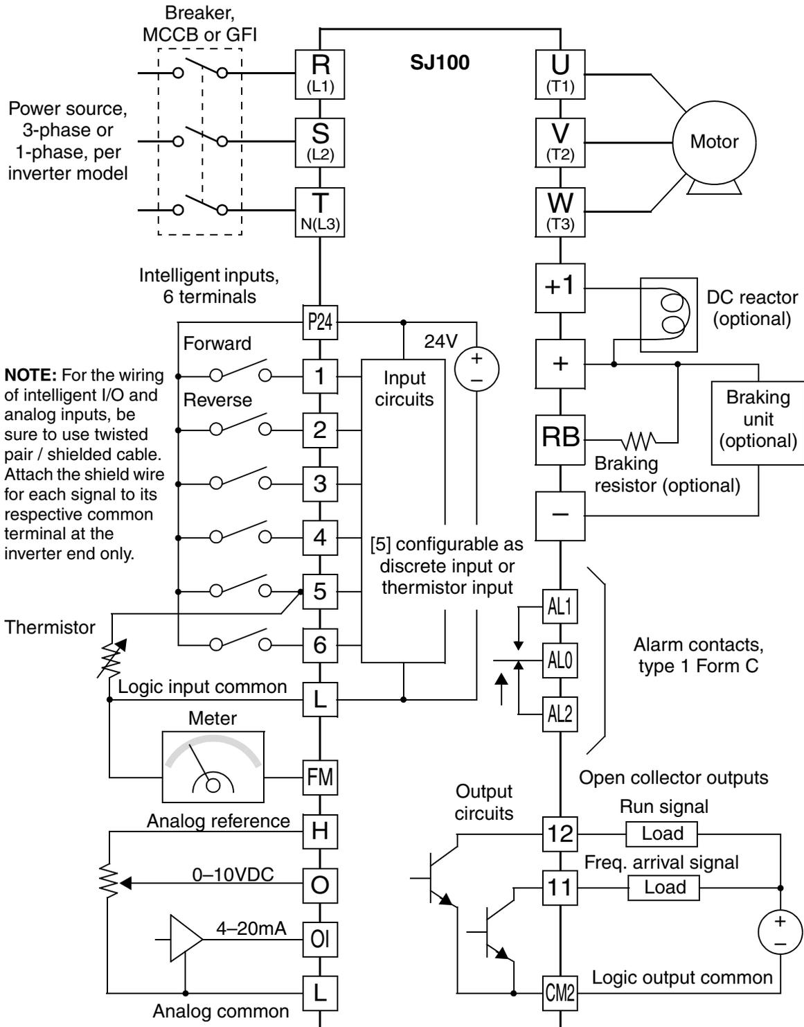
**NOTE:** For the wiring of intelligent I/O and analog inputs, be sure to use twisted pair / shielded cable. Attach the shield wire for each signal to its respective common terminal at the inverter end only.
